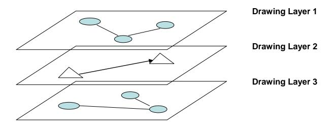
Each drawing layer can contain any number of drawing elements, which have to be instances of the interface IDrawingElement.
